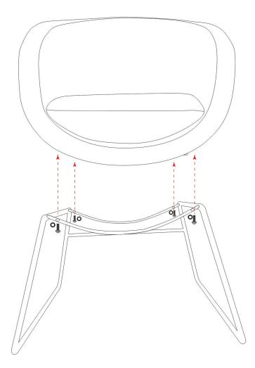
Use the screws and washers provided to attach the frame to the underneath of the seat base as shown
