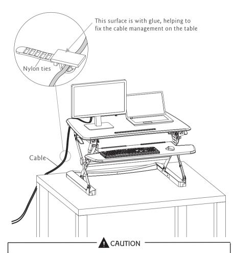
Adhesive buckle helps to make the cables tidy and cleanPlease leave enough length of cable for height adjustment function, otherwise it may cause unexpected lost.
