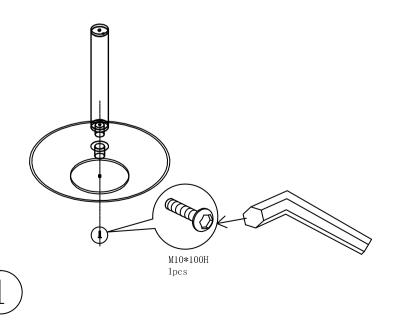
Step 2. Attach top disc to top of the pole
